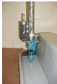
The Drop Dart Test ensures impact resistance ductility.
